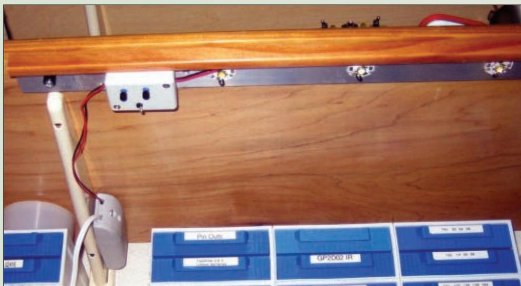
Figure 8. Workbench light with PWM dimmer.
