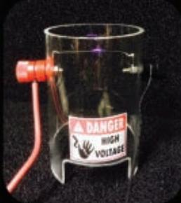
Plasma is a hot ionized gas that is electrically conductive. The plasma arc speaker creates a plasma using a high voltage electrical discharge. When an audio signal is passed through the plasma it causes it to vibrate in sync with the audio signal. The plasma in turn vibrates the air around it to create sound.
